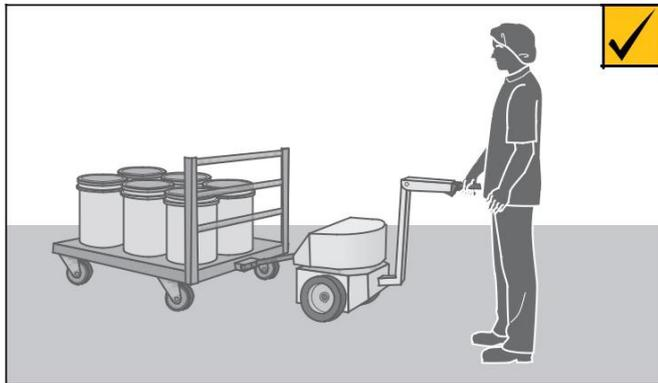
Use a tug (shown), conveyer or scissor trolley to allow workers to work in appropriate postures without exerting excessive force.
